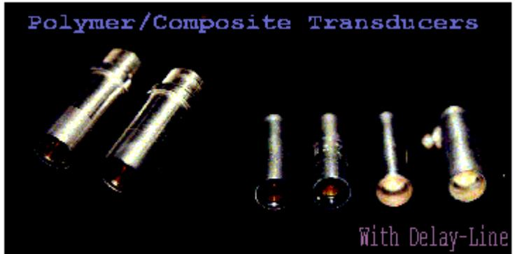
Since the polymer withstands higher voltage than ceramics - even 50MHz transducer has an electrical strength of 1KV or more - it is possible to use a pulser with higher transmitter voltage for excitation of ultrasounds. In this case, the total gain of polymer transducers will be much higher than ceramics transducers.
